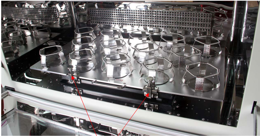
The claw-like platform safety latches
