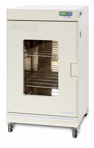
The drying oven can store 9 programs 18 steps in memory. Steps can be set for running multiple "ramp and soak" cycles, or for just running at one temperature for a given time and then switching automatically to another temperature for another given time. Each program can be made to repeat from 1 to 99 times automatically.
