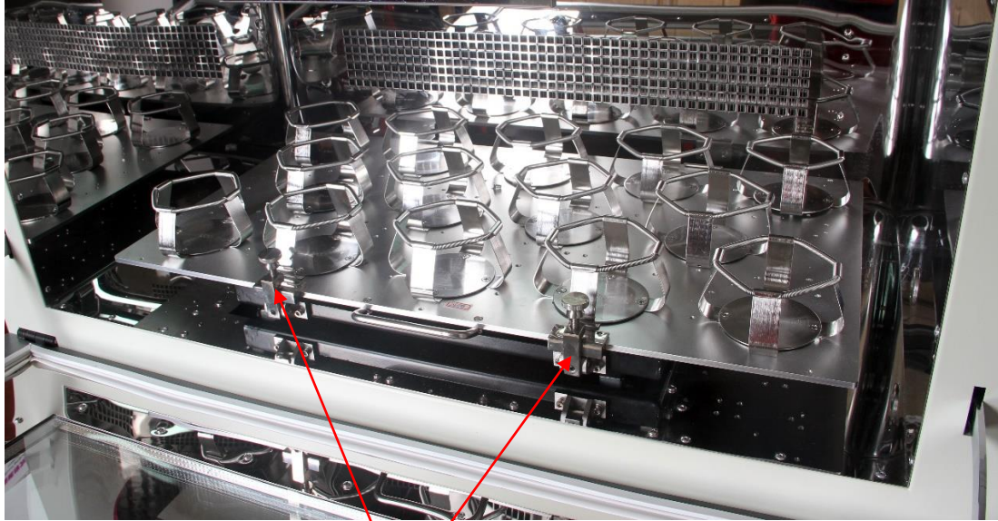
The claw-like platform safety latches
